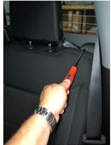
Using a small hook tool reach in behind the lean back hooking the latch mechanism and lifting up to release the lean back from the wall. Once the lean back is released from the back wall place a wedge between the lean back and the wall to prevent it from relocking. Repeat same process for the two remaining locking mechanisms.
